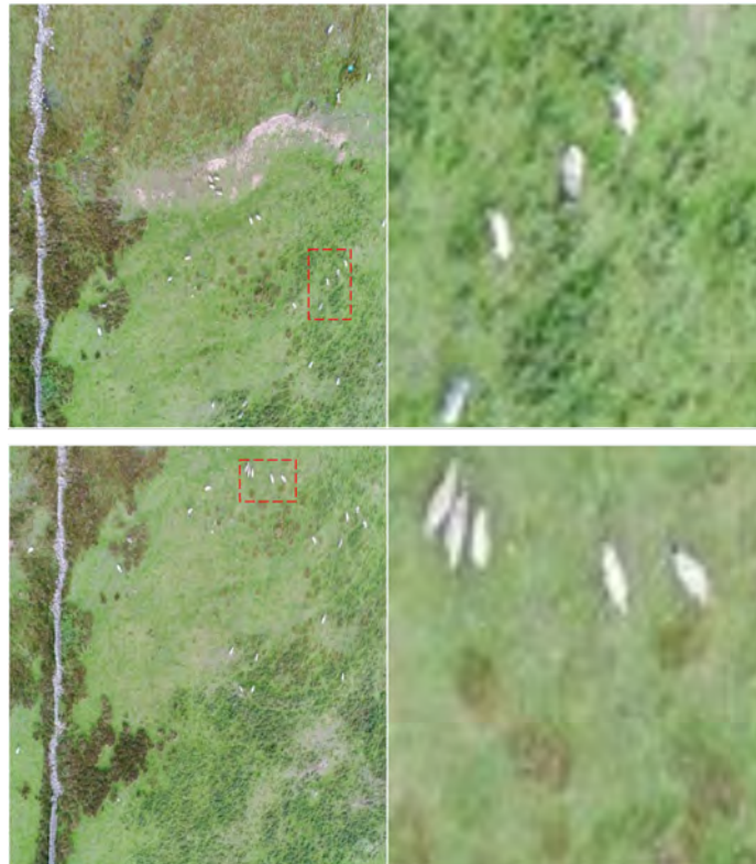
Figure 7. Images of livestock captured from a UAV at 50m altitude. Left column shows the original images. The right column images zoomed versions of the livestock targets. At high altitudes, livestock are captured as small target objects in the images.
