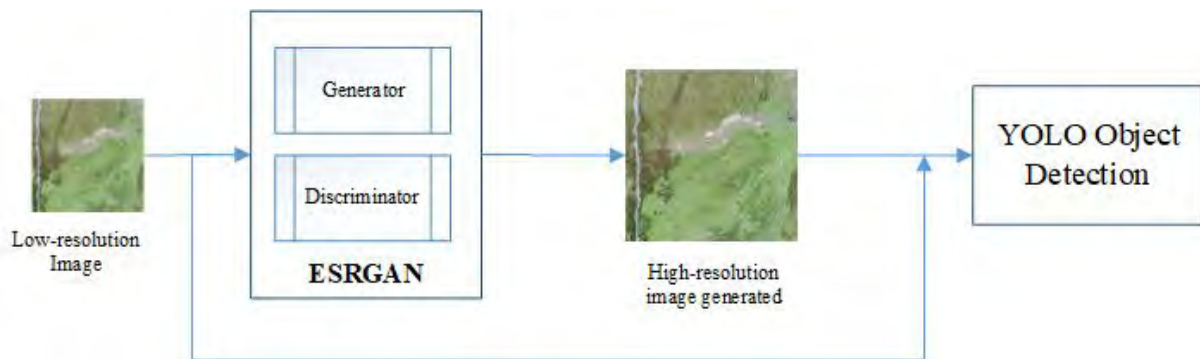
Figure 8. The ESRGAN and YOLO object detector based system used in our study to generate super-resolution images for small object detection on livestock images.
