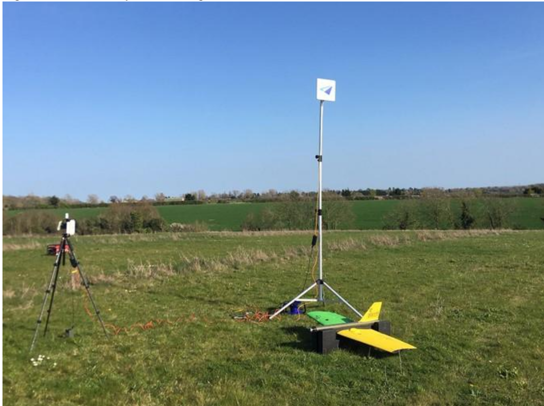
Figure 8: Blue Bear's ground station connected to 5G with the Agristart fixed wing
