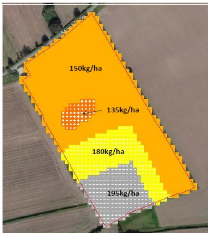
Figure 5. Prescription map for seed rate application based on previously captured drone imagery.
