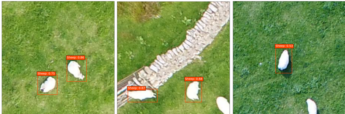
Figure 5. The detection results obtained from the SSD algorithm. The red bounding boxes indicate the detection performed on the split aerial images.
