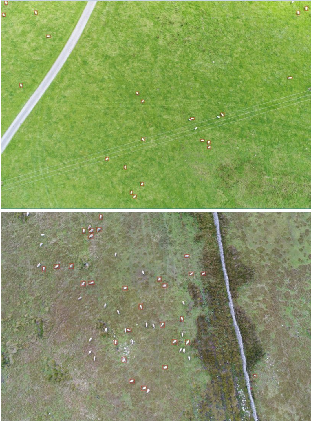
Figure 7. Livestock detection results obtained by the extended SSD algorithm. The red bounding boxes on the sheep illustrates the detection performed by the algorithm.
